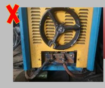
Electrical equipment terminal box without proper cover
